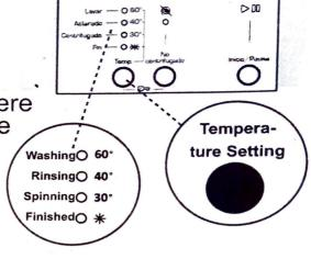
You can gradually decrease the washing water temperature between the maximum washing water temperature of the selected programme and cold washing \*\* selections by pressing temperature adjustment button.
