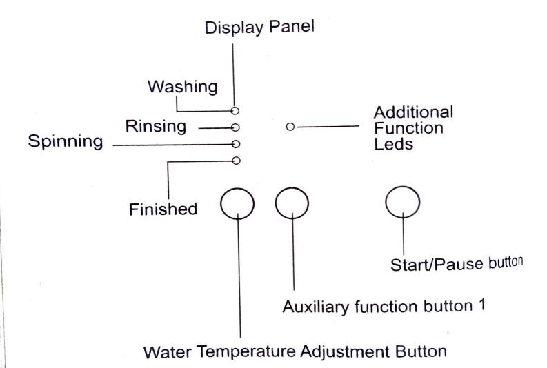
From the function leds of your machine, the washing water temperature of your machine, the auxiliary functions you have selected and the stage of the programme you are running on your machine. up pre wash / wash state, rinsing stage, spinning stage).
