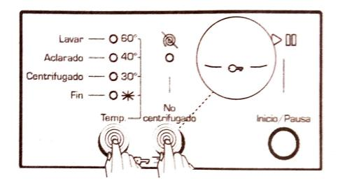
If pressed any button while child lock is active, the Additional Function Leds will blink on the display.
